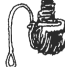
Wind rope-tail around bundle (two circuits makes it more secure) and tuck through itself
